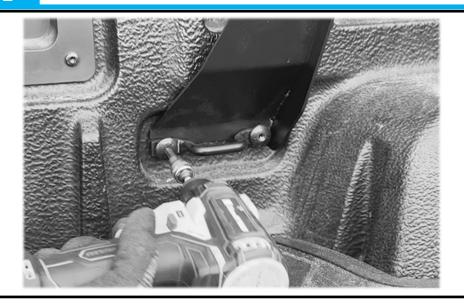
Install the front mounting brackets [1] in place of the hooks. Reuse the existing bolts or alternatively using the provided fasteners:
