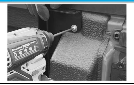
Bolt the bracket to the side of the tub reusing the existing fasteners or using the following provided fasteners:
