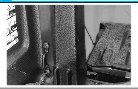
Install the rear mounting brackets [2] in place of the hooks. Reuse the existing bolts or alternatively using the provided fasteners:
