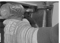
Remove the bolts fixing the small rear brackets in place
