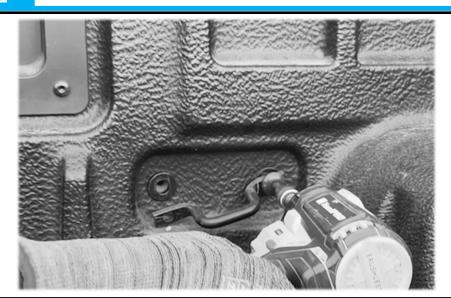
Remove the central tub hooks on both sides
