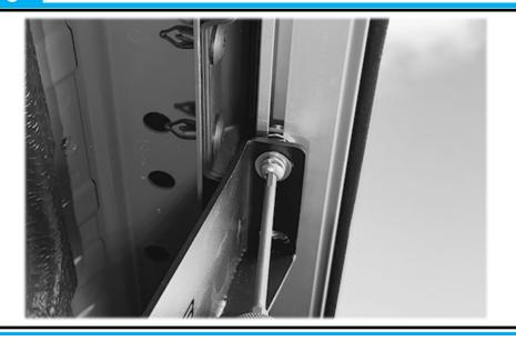
Bolt the front mounting bracket to the T-Track and flange nuts using the following fasteners:
