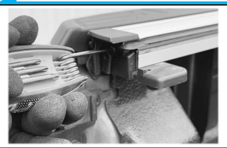
Remove the rubber capping at the rear of the roller lid track
