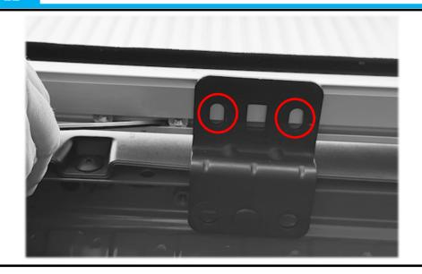
Slide the flange nuts down the t-track so that there is one nut over each hole in the mounting brackets.
