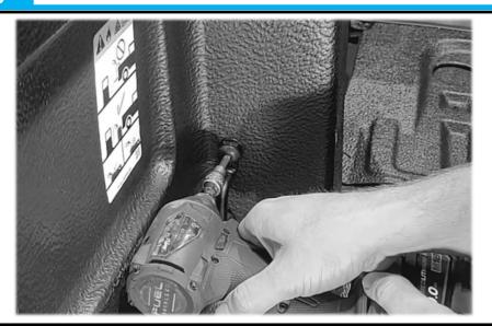
Remove the rear tub hooks
